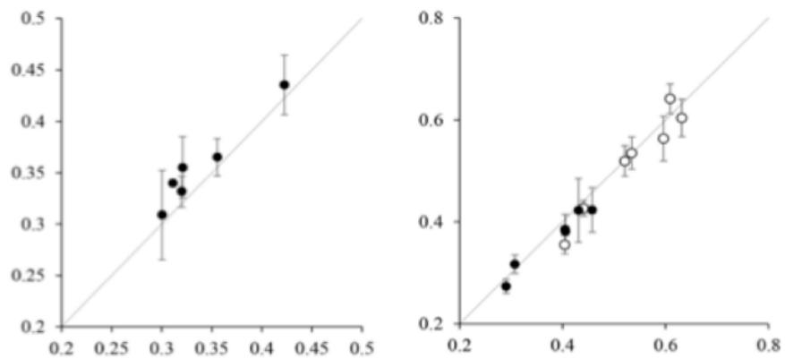
Fig. 3 Comparison of the depth of the upper fresh-saline interface and the lower particle-laden - particle-free interface in terms of the model prediction and the experimental measurements obtained from the images (after Mingotti and Woods 2015).
