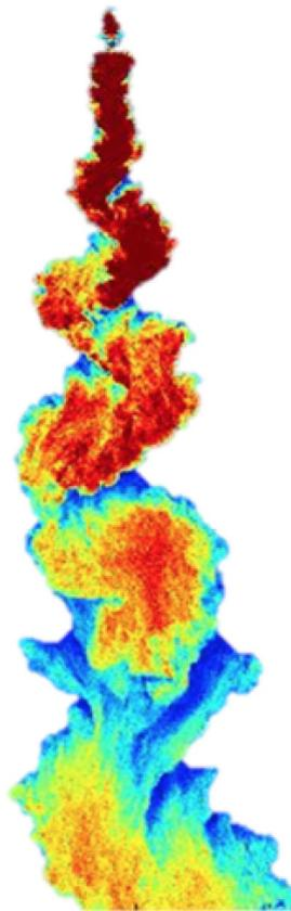
Fig. 4 Image of the salinity structure in a turbulent two dimensional plume, showing how the mixing leads to a gradual dilution of the flow and also that there is a considerable level of stratification in the flow associated with the turbulent eddies.
