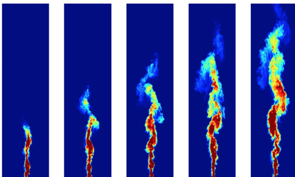
Fig. 5 Image of the evolving tongue of dyed fluid migrating into the plume further downstream in the tank. This data can be used to predict a dispersion coefficient for the mixing (see Rocco and Woods 2015).
