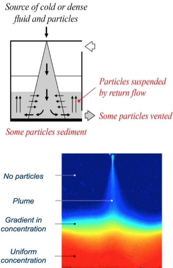
Fig. 1 Particle profile produced using light attenuation in the case of a plume of particle laden fluid descending into a ventilated reservoir. The reservoir is ventilated in the downwards sense. The layers observed in the figure correspond to a particle rich layer in the lower part of the vessel, and a particle free layer higher in the vessel.
