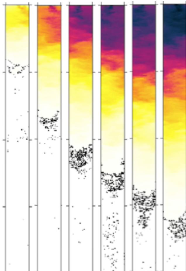
Fig. 6 Series of images showing the advance of a continuous source of saline water supplied to the top of a tank. The images, at equal time intervals, illustrate the gradual increase in salinity at the top of the tank and also the gradual slowing of the advancing front with time, as expected for a self-similar deepening of the saline region.
