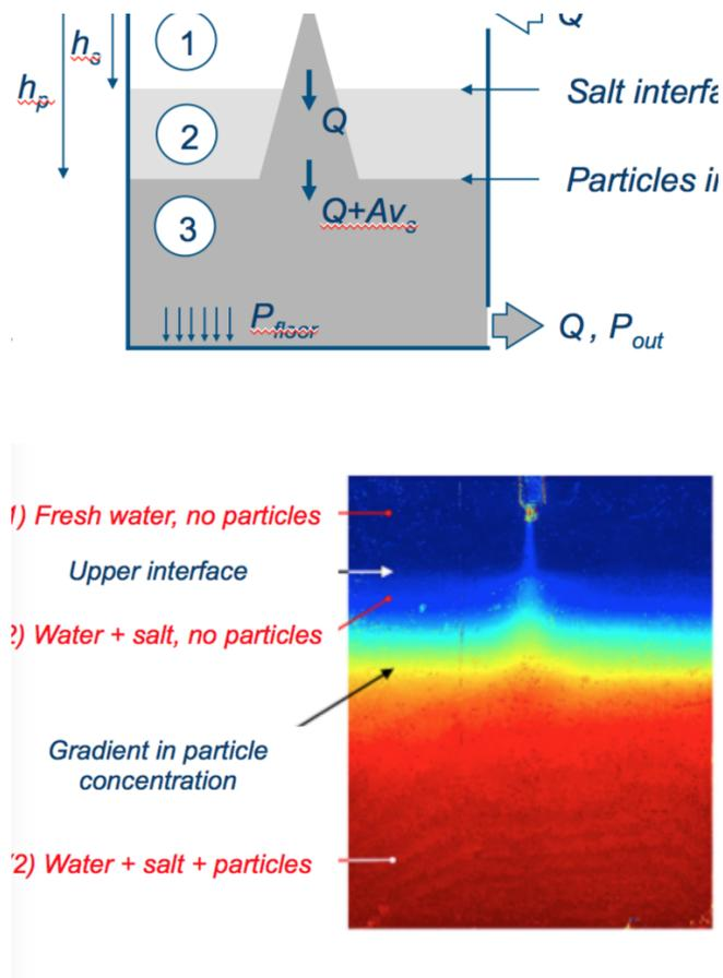
Fig. 2 Variation of the light intensity in the case of a particle laden plume of saline water flowing into a downward ventilated vessel. In this case three layers develop in the system. A fresh water layer, a saline layer and then a particle laden saline layer. After Mingotti and Woods 2015
