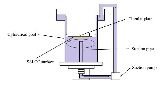
Fig. 3 Schematic view of test section system for vortex suction flow experiment
