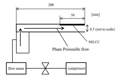
Fig. 2 Schematic view of preliminary experiment system
