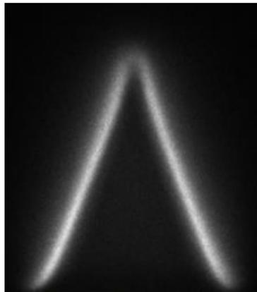
Fig 3. Instantaneous photography of flame front of methane at equivalence ratio  $\phi=1.0$
