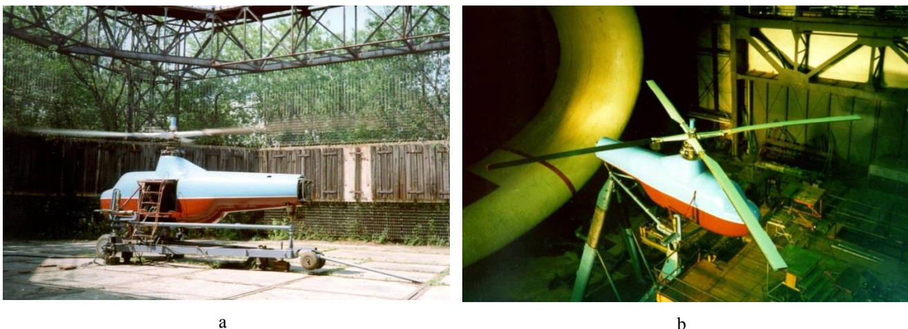
Fig. 10 Measurements of motion and deformation parameters of helicopter rotor blades on the hovering (a) and in the T-101 wind tunnel (b)
