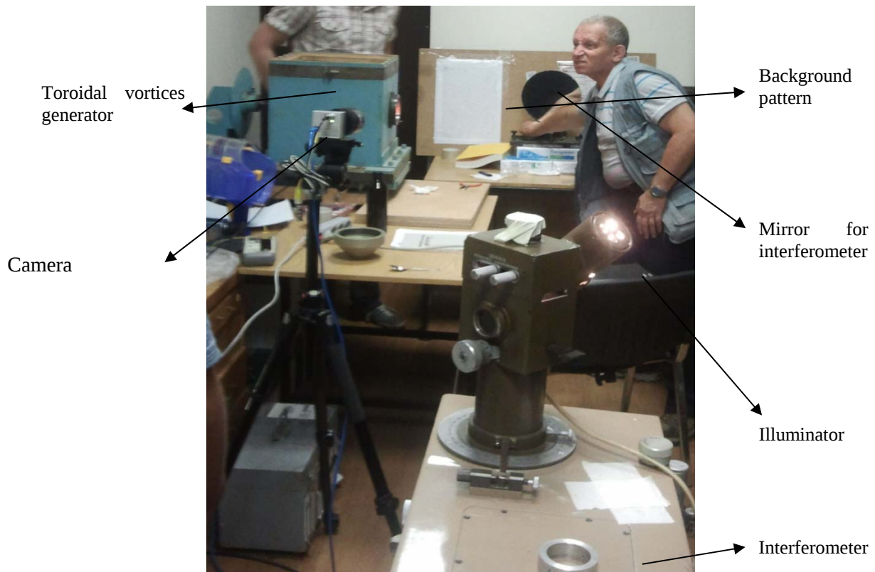
Fig. 3 The part of experimental setup for realization Background Oriented Schlieren method
