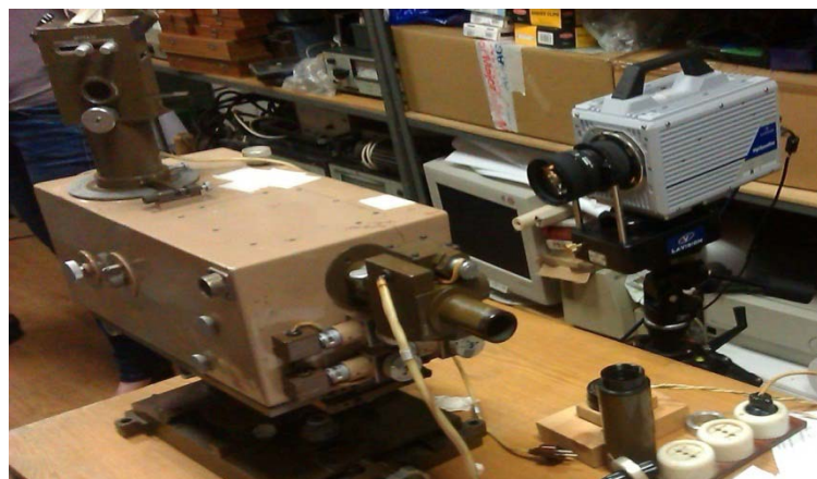
Fig. 3 The part of experimental setup for realization Background Oriented Schlieren method
