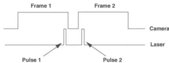
Fig. 2 Straddle time between pulse 1 and pulse 2
