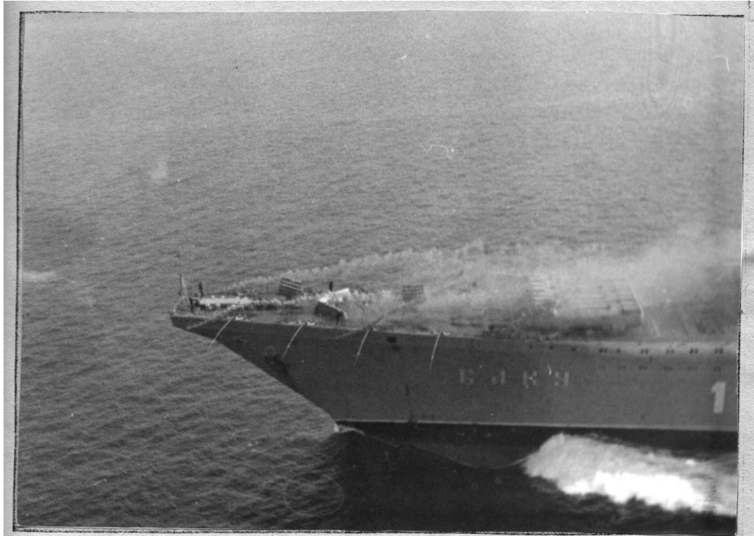
Figure 4. Visualization of nose part of AC overflow. Side view.
