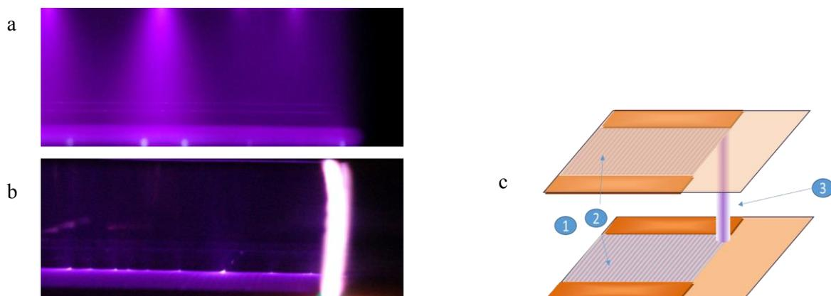
Fig. 2. Two regimes of combined discharge (a, b) and the scheme of plasma column formation (c). 1 - discharge volume, 2 - plasma sheets, 3 - contracted volume discharge (plasma column).
