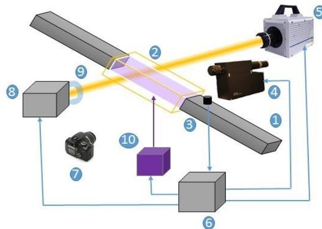
Fig. 1 Experimental setup: 1 - shock tube, 2 - discharge chamber, 3 - pressure gages, 4, 5 - high-speed cameras, 6 - delay generator, 7 - photo camera, 8 - light source, 9 - optics, 10 - spark-gap controller
