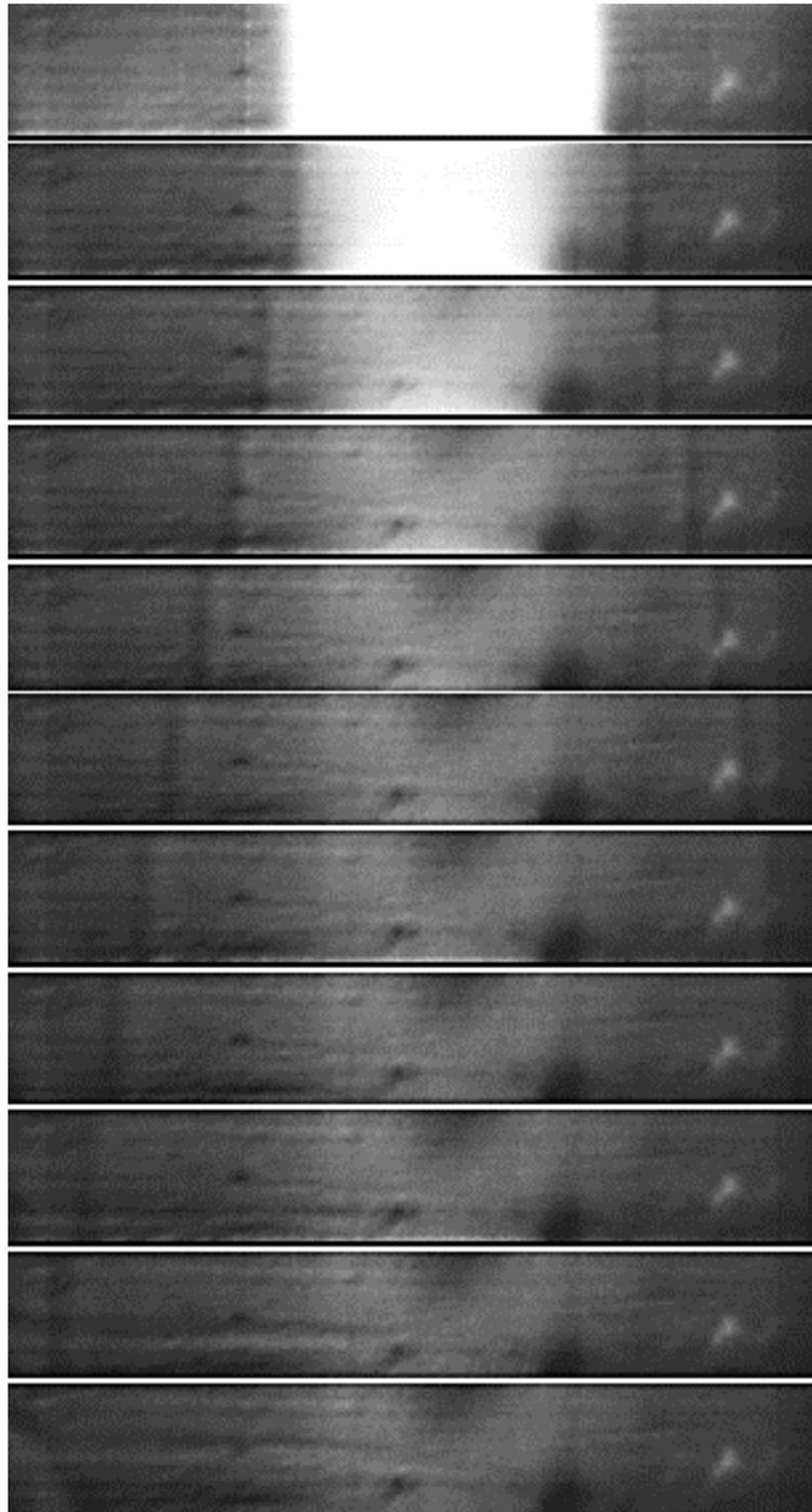
Fig. 5. Sequence of 11 shadow images of shock configuration from the discharge channel, taken with a frame interval of 1.9  $\mu$ s at a pressure of 120 Torr.
