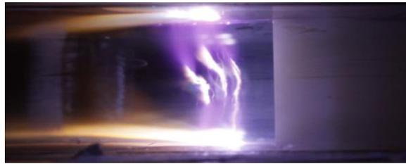
Fig. 6. Glow image of controlled discharge localization in low density area. Flow from right to left.
