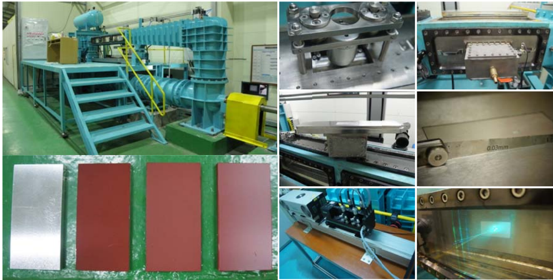
Fig. 4 Photos of the high-speed water tunnel, flush-mounted balance and the samples of FDR-SPC and FDR-AF coatings
