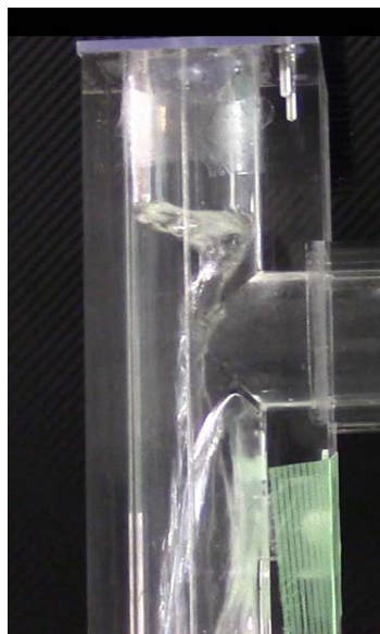
Fig. 6 Visualized intermittent vortex tube in side view
