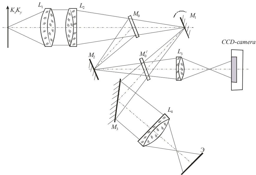
Fig. 2 Shear interferometer scheme
