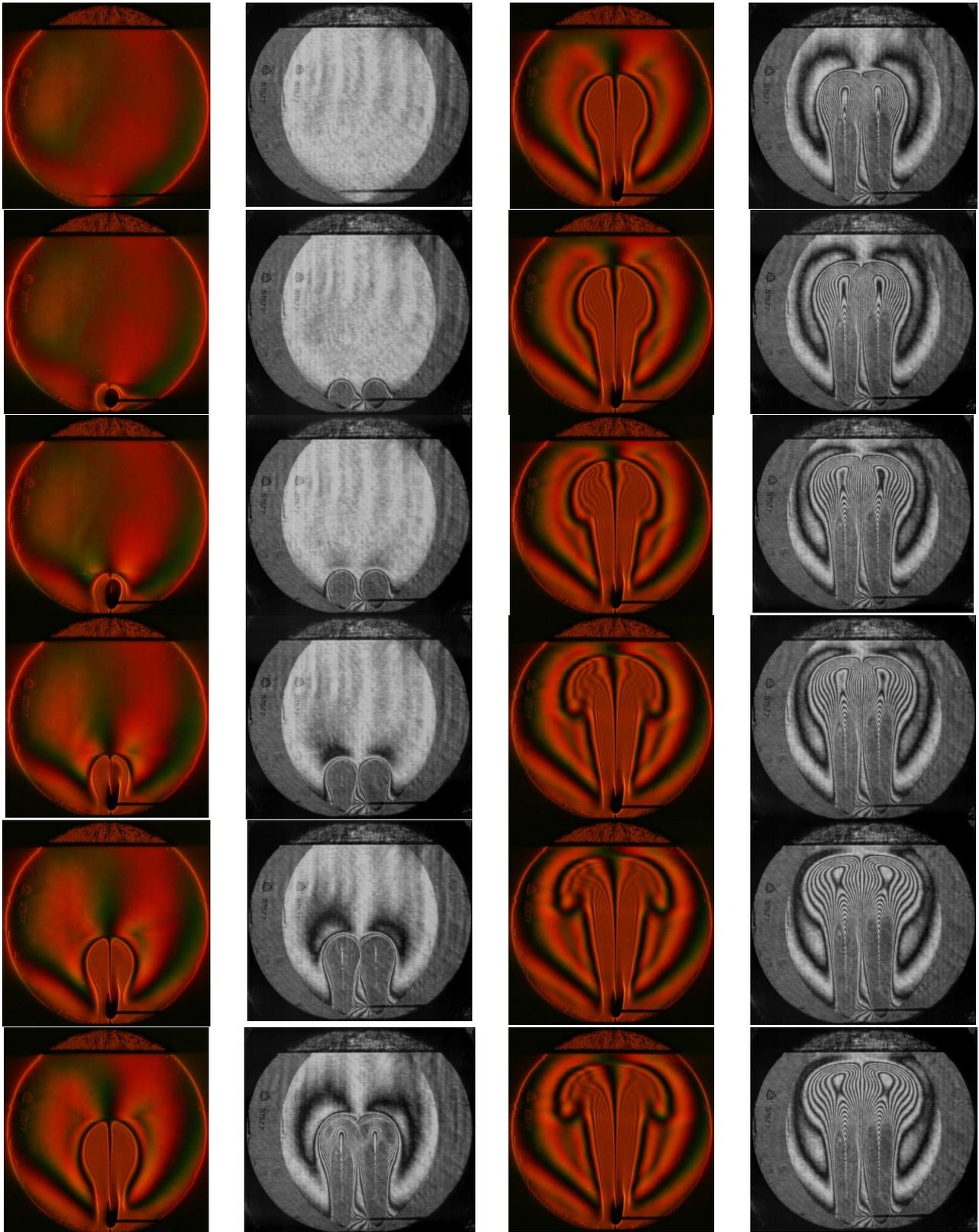
Fig. 3 Sequence of Hilbert and shear interferogram images of the plume
