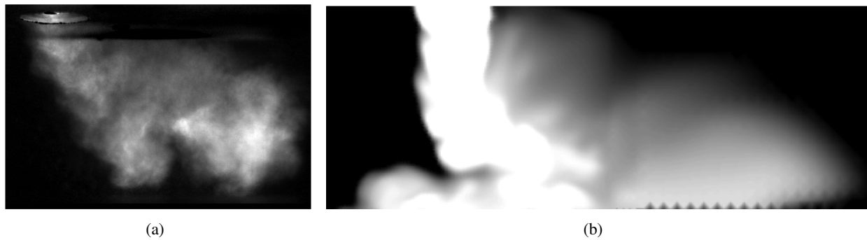
Fig. 5 Example images for the case of MR = 0.59 , (a) Experiment, (b) CFD result.
