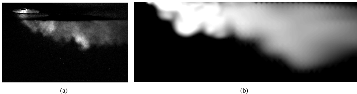
Fig. 6 Example images for the case of MR = 7.54 , (a) Experiment, (b) CFD result.
