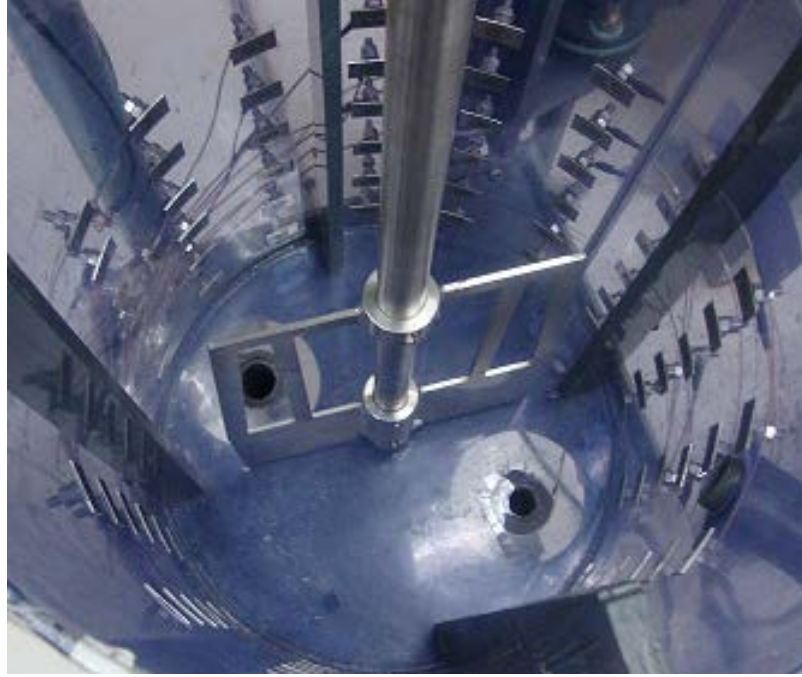
Fig. 3 Tomography electrodes installed on the periphery of the mixing tank.
