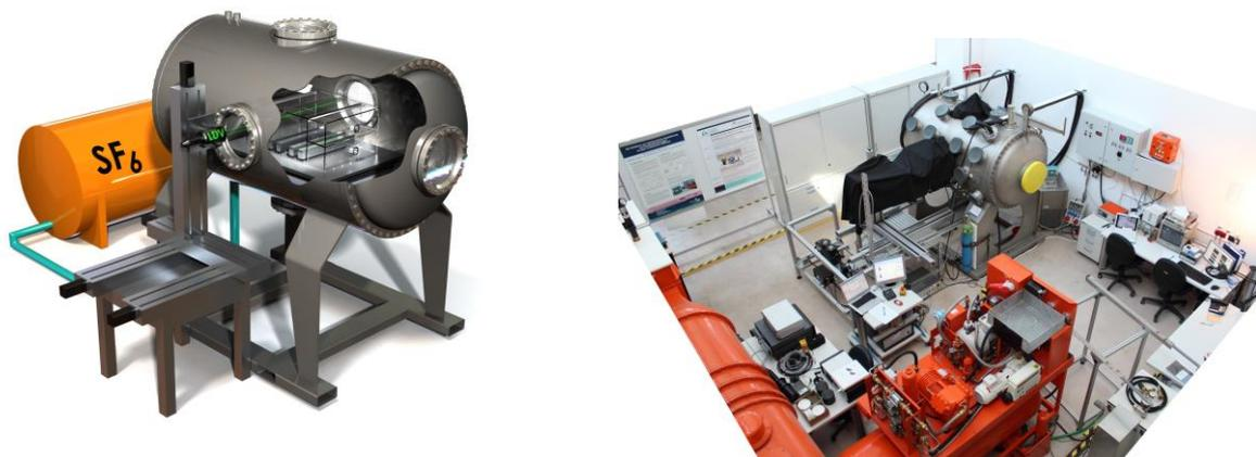
Fig. 1 Sketch of SCALEX (left) and picture of the whole facility (right). The pressure vessel of 2m x 1.m dimension works with pressurized SF<sub>6</sub> up to 10bar. The size of the model cell is limited to 0.75m x 0.5m x 0.5m. The pressure vessel is connected with a SF<sub>6</sub> storage system (orange part in right picture).
