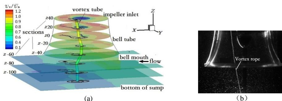
Fig.8 The developing of the vortex rope in the pump intake under large flow rate(1.2Q0)
