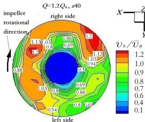
Fig. 5 Axial velocity  $v_z/\bar{v}_z$  distribution of Impeller inlet section
