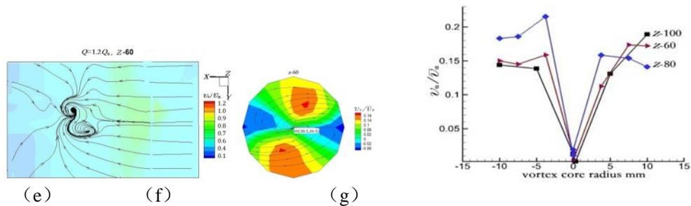
Fig.7 The axial distribution, streamlines of the sections below bell-mouth and tangential velocity distribution in vortex cores
