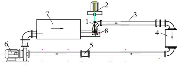
Fig.1 Vertical axial flow test loop
