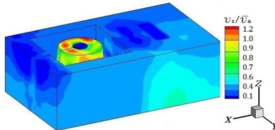
Fig.4 3D-volume flow field of the pump intake
