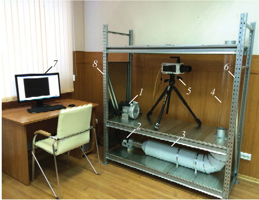
Fig. 1 Experimental setup: 1 – air fan; 2 – air heater; 3 – heated air supply channel; 4 – hollow glass cylinder; 5 – high speed video camera; 6 – yardstick; 7 – computer; 8 – control panel
