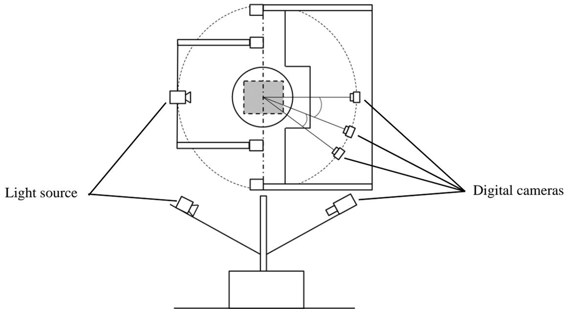
Fig. 1 Layout of experimental apparatus
